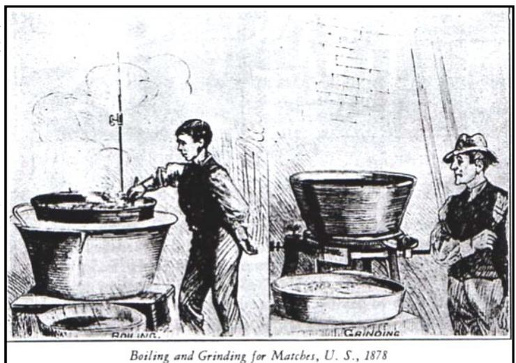
Boiling and Grinding for Matches, U. S., 1878
